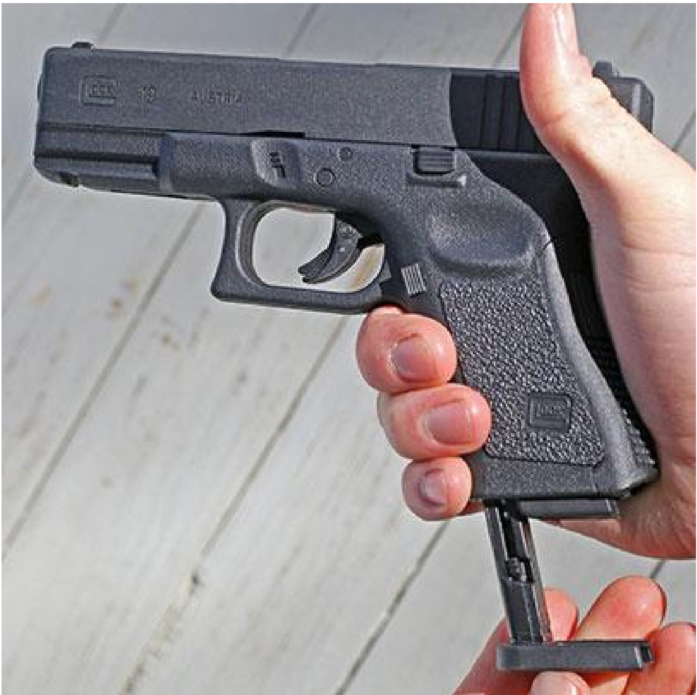
The 15-round magazine of the Umarex Glock 19 Gen 3 fits into the grip just like a conventional magazine and is released by a magazine button in the same position as that on a centerfire Glock 19.
